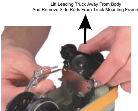
Figure 8: Lift Truck Away From Body To Reveal Headlight
