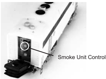
Smoke Unit Control
