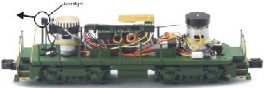
Figure 6. Replacing the Light Bulbs
