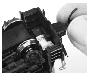
Line Up CENTER Mounting Hole In Coupler Pocket With Mounting Hole On Chassis
