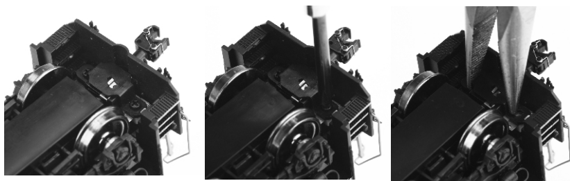
Identify & Remove Mounting Screws
